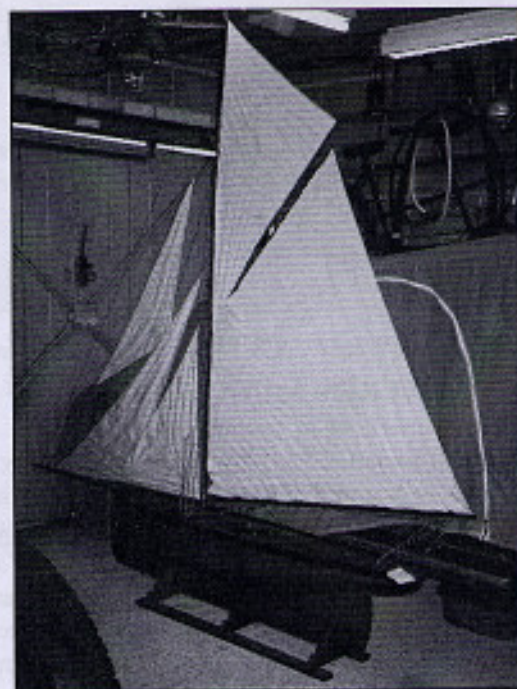
A very large straight stemmed Gaff Cutter similar to those sailed on the Serpentine. Some idea to the size may be gained by comparison to the 2m high garage door in the background.
